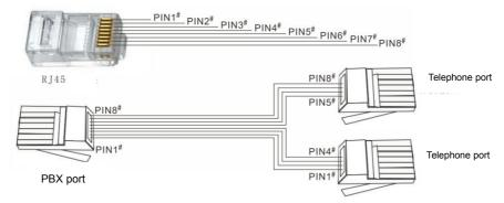
When user need to lengthen the cable or make a 4 wire cable by himself, he should be attention to the sequence of cable: the two wires on middle are signal line . Pin1 and pin4 are data line. If wrong connection, the key phone will not work. Furthermore make sure good contact and correct line sequence when make the RJ11 crystal connector.
